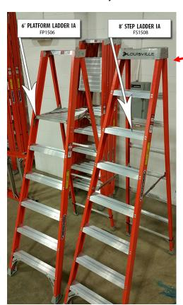
Note a 6' Platform ladder is a 6' working height vs. an 8' Step ladder which has a 6' working height.
